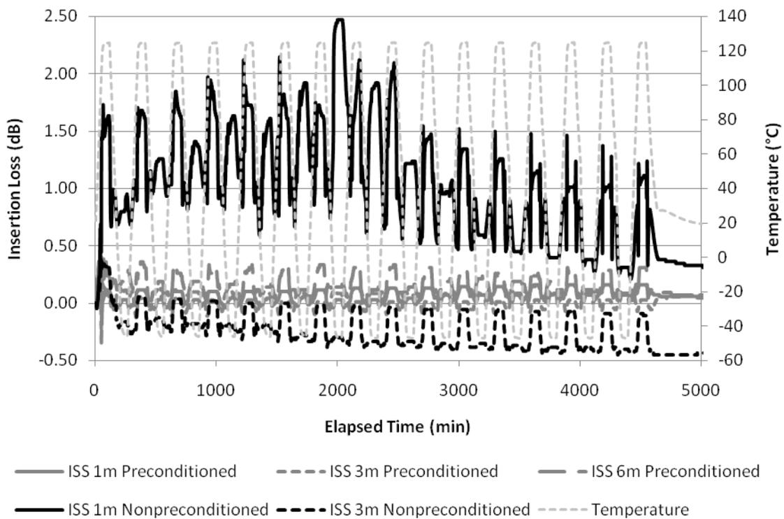
**Figure 10: Comparison of insertion loss versus temperature for preconditioned and non-preconditioned International Space Station (ISS) cables measured at 850 nm.**
