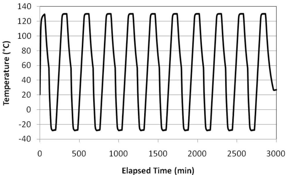
**Figure 3: Temperature profile for fiber optic cable preconditioning.**
