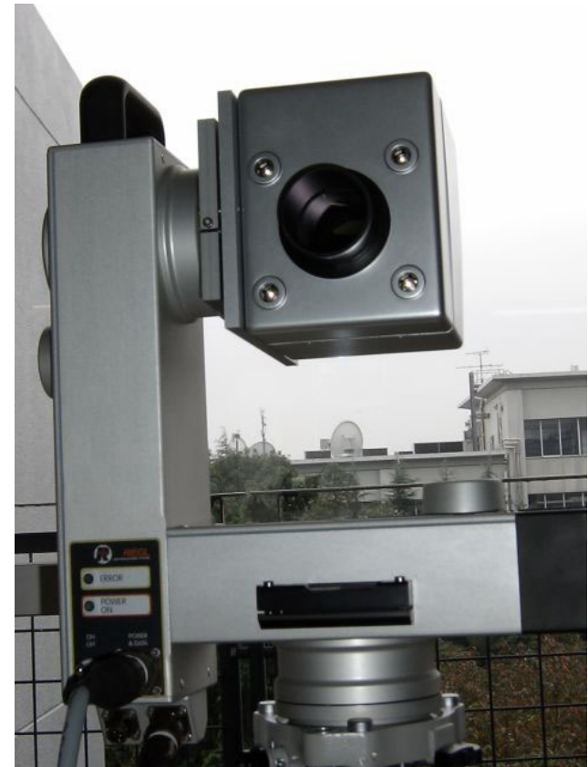
External view of antenna module and two-axis gimbals
