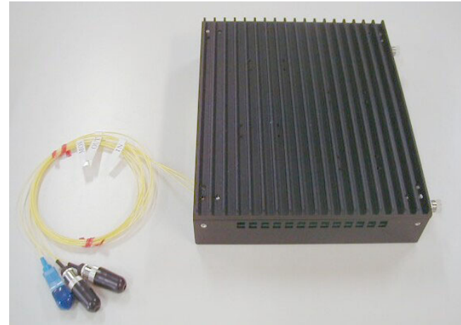
Gain unit for high power Er-doped fiber amplifier
