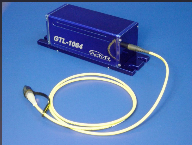
Prototype pulsed SLM 1064 nm seeder TRL 4-5
