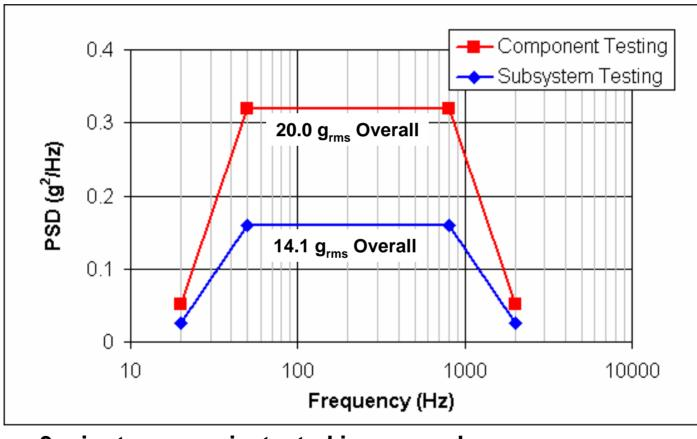
3 minutes per axis, tested in x, y, and z.
