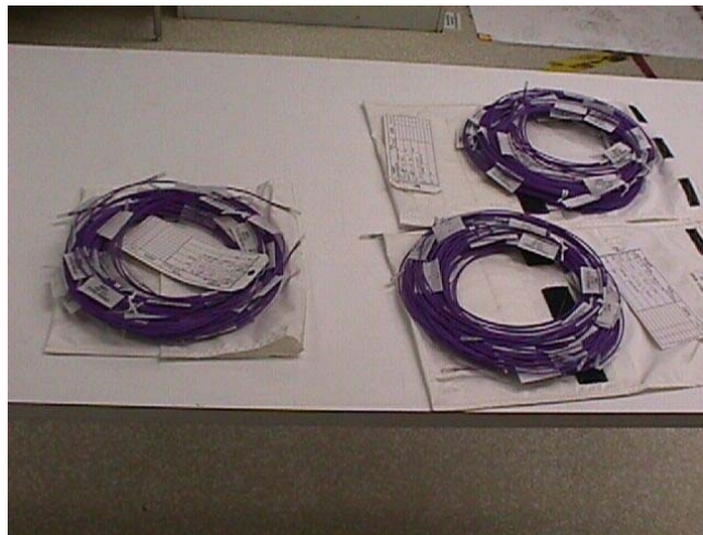
Terminated Flight Links (QTY 36 in 12 Configurations stored In four different low level softpacks)
