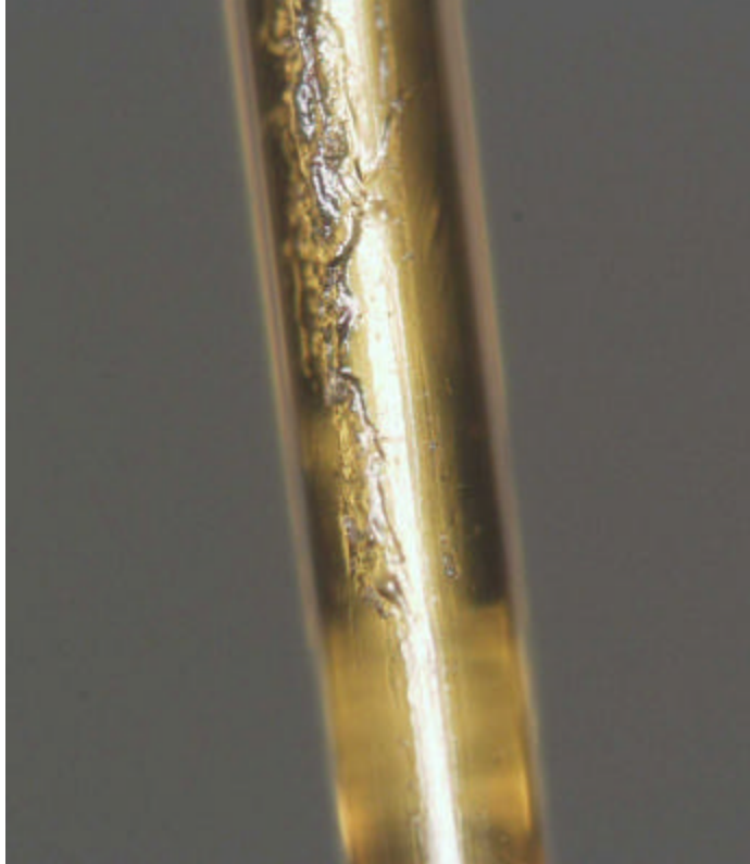
Typical “under curing” (post application reflow)
