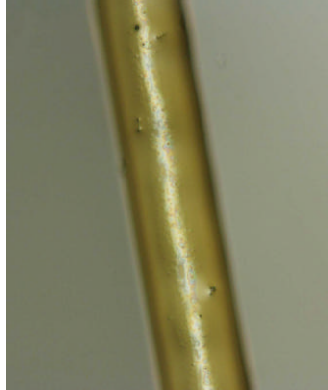
Typical “blistering” (inadequate cure between coats)
