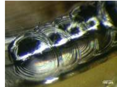
Solder joints for the output optical pigtail
