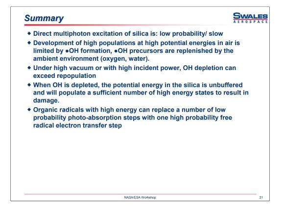
Irradiation of glass by radiation from sources such as UV, x-ray, gamma, electron and laser irradiation affects glass in relation to the radiation absorbed dose (RAD). This dose will result in changes in the physical and chemical properties of the glass. Population of elevated energy states occurs through the population of metastable states in the glass. Including the softening of the glass.
