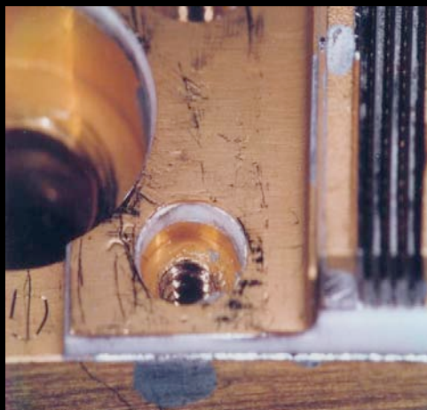
Indium creep onto the gold wires Intermetallic Gold/indium
