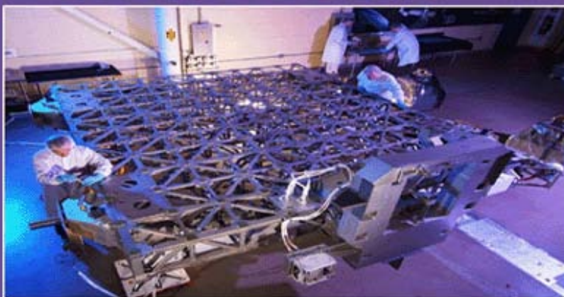
Engineers inspect one of the ExPRESS Logistics Carriers in the small clean room at NASA's Goddard Space Flight Center
