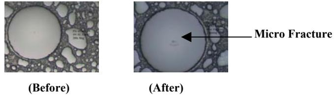
Figure 4: Image Inspection Before and After Vibration of Cable Config-B-1
