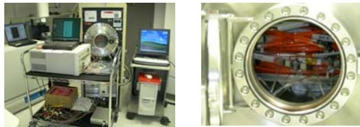
Figure 6 & 7: Thermal Vacuum Setup and Cables Inside Chamber
