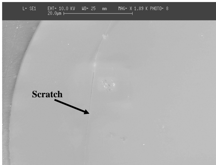
Figure 7.7-4. Scratch at Magnification of 1.89 \times 10^3 \times
