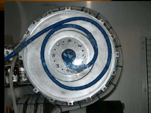
Window inside gimbal; Bundle cable inside.
