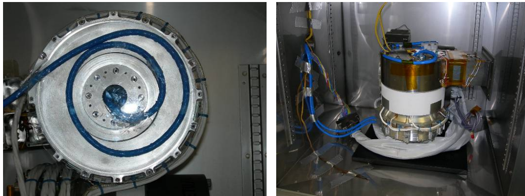
Figure 7a) Gimbal in loose position, b) Inside the Thermal Chamber, Gimbal with Fiber Bundle Integrated.
