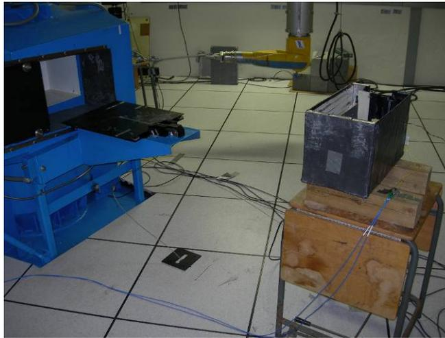
Figure 3: LiNbO<sub>3</sub> Modulator in radiation test cell
