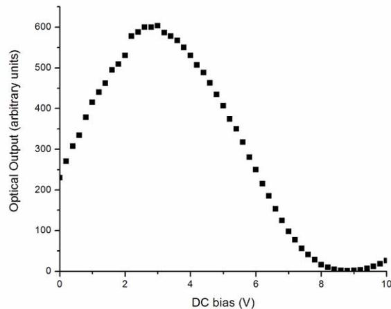
Figure 4: DC bias versus optical output from modulator with no RF bias applied
