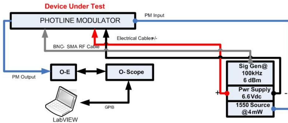
Figure 1: Modulator experimental setup
