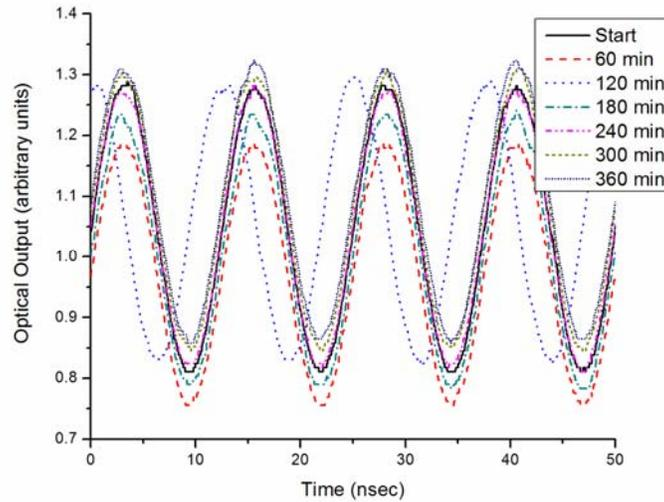
Figure 8: Modulator output after radiation test. Data were collected a month after completion of radiation test. Drift in output is similar to pre-irradiation results. No change in frequency or peak-to-peak output was observed.
