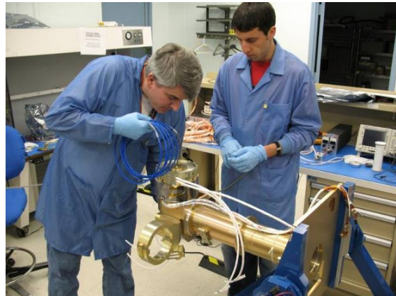
Figures 11 a) FOB 2 being routed into the cable wrap on gimbal 2, b) Photonics Group members, Richard Chuska and Robert Switzer work on integration of the FOBs to the gimbal cable wraps.
