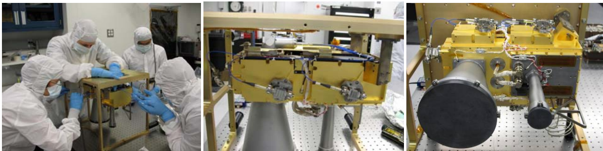
Figure 6 a) LOLA flight integration team, including Lead Mechanical Engineer Steve Schmidt, Lead Fiber Optics Engineer Melanie Ott, Quality Assurance Engineer Keith Cleveland, and Optical Engineer Robert Switzer, b) side view of two detectors that were coupled to two channels of the fan out side of the optical bundle assembly, c) LOLA instrument fiber integration complete.
