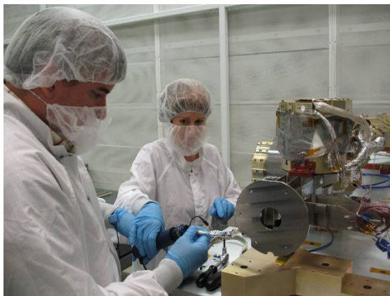
Figures 12 a) Richard Chuska and Melanie Ott conduct transmission testing on FOB 2 with gimbals now attached to the entire boom arm, b) Melanie Ott and Adam Matuzeski integrate the FOB 2 to a safe position after integration down the boom, while awaiting the mandrel installation.
