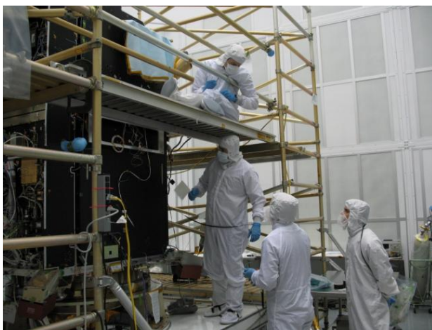
Figure 15 a) William Joe Thomes on second level scaffolding and Richard Chuska routing behind where HGAS will be stowed for launch, b) William Joe Thomes performing FOB 3 routing on the early morning shift before space craft operational testing begins for the day.
