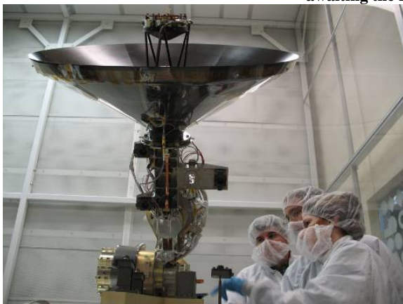
Figure 13a) The team investigates - the full motion of the High Gain Antenna comes close to the optical cable routing configuration. B) Richard Chuska motions that the High Gain Antenna is now fully integrated to the gimbals and boom arm.
