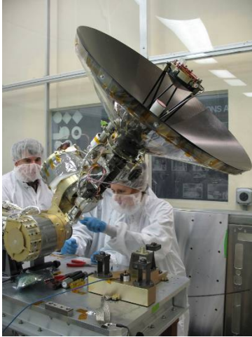
Figure 14: a) Richard Chuska, Adam Matuzseski and Melanie Ott watch the motion of the HGA with gimbals running through their full range of motion, b) Melanie Ott routing FOB 3 under the Instrument Module deck
