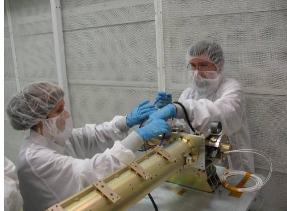
Figures 12 a) Richard Chuska and Melanie Ott conduct transmission testing on FOB 2 with gimbals now attached to the entire boom arm, b) Melanie Ott and Adam Matuzeski integrate the FOB 2 to a safe position after integration down the boom, while awaiting the mandrel installation.
