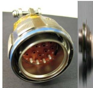
Figure 18: MIL-SPEC-38999 connector and 29504 termini.
