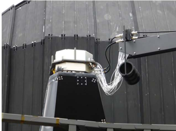
Figure 2. JWST testing of the combined OTE and ISIM to form OTIS. Optical stimulation is provided by ASPA located at the intermediate focal plane of the OTE. ASPA fiber optics was a collaboration of NASA GSFC and Ball Aerospace.
