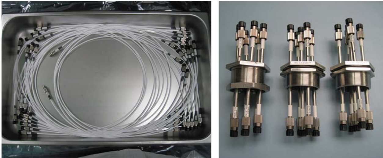
Figure 4. Fiber assemblies from OSIM interface plate for linking to the vacuum fiber feedthroughs. Custom fiber vacuum feedthroughs for interfacing to the SES chamber. All assemblies and feedthroughs manufactured by GSFC 562 Photonics Group.
