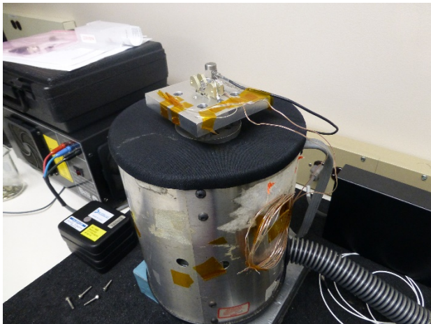
Figure 1: ATLAS Q-Switch vibration test in GSFC Photonics Group environmental test lab.
