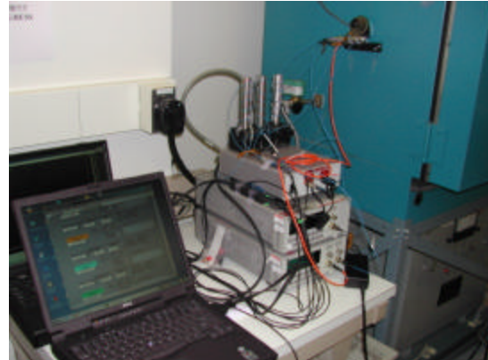
Figure 5a) Mated Pairs Inside of Thermal Chamber, 5b) Experimental Set up Used for Monitoring Optical Power During Testing
